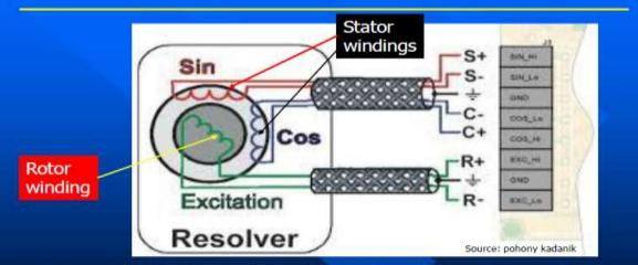
Rotor winding is rotating with the load and is excited by AC input voltage.
